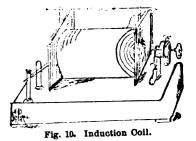
It consists in fact of two coils of wire, one within known as the primary coil, directly connected with the battery, and an outer coil having no electrical connection with the other or with the battery, and known as the secondary coil. Whenever a current is started or stopped
